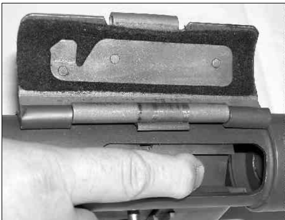
Above: Charging the Carbine is accomplished similar to the original M3A1 Grease Gun. A finger must be inserted into a slot in the bolt, and the bolt pulled rearward. Unlike the original SMG, this new semiautomatic version fires from a closed both.
