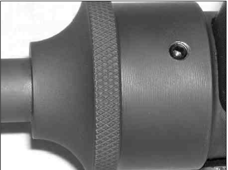
The barrel can be removed for cleaning or replacement by simply loosening this allen screw and turning the knurled barrel nut counter clockwise.
